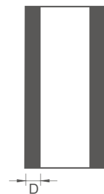
Thickness of copper pipe
