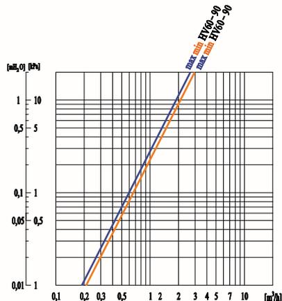
**Colector 2m³/h - 50Kw - SG**
